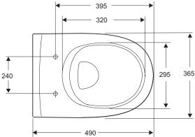
All measurements shown are in millimetres. Sizes are approximate.
